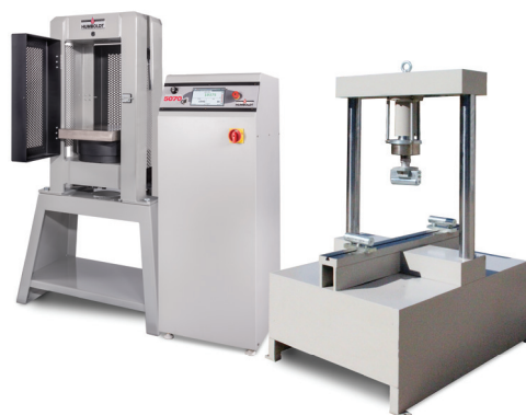
HCM-1144 Flexural Frame and a concrete compression machine controlled with a HCM-5070 Console Automatic Pump and Controller System.
